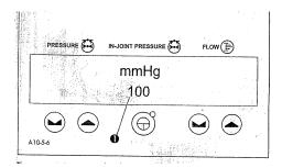
The pressure is measured at the pressure chamber. The in-joint pressure display is calculated by means of the measured pressure and the following operating parameters:
