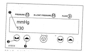
Select the desired pressure. The desired pressure display shows the preselected value 10 in mmHq.
